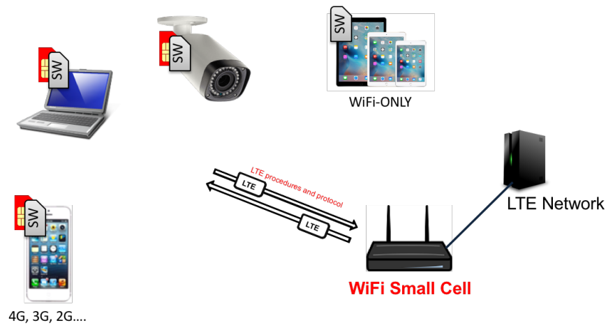
Figure 8: LTE-WiFi convergence platform connecting any device
